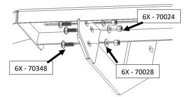
Figure 1: Bolting Mounting Blades to Nerf Step
